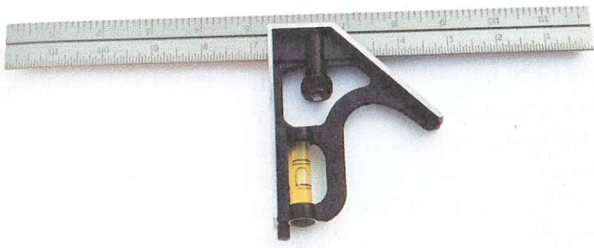
FIGURE 11-5 The body and blade of a combination square are adjustable.
