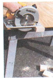
FIGURE 14-4 Saw cuts are made over the end of supports so that the waste will fall clear and not bend the blade.
